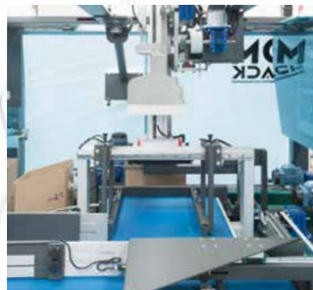
New generation case packer machine, unique. Compact, automatic, simple in the change of format and adjustments (all motorized).
