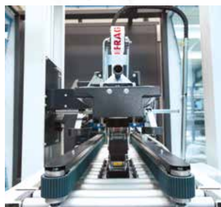
Out feed station with motorised driven belts adjustable for different carton sizes.
