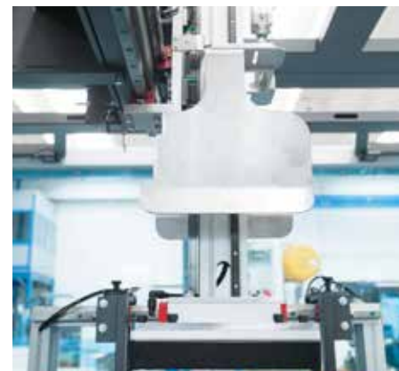
Pick and place for fast & accurate products picking up from the in feed transport conveyor and precise feeding of the carton with the configuration previously set.
