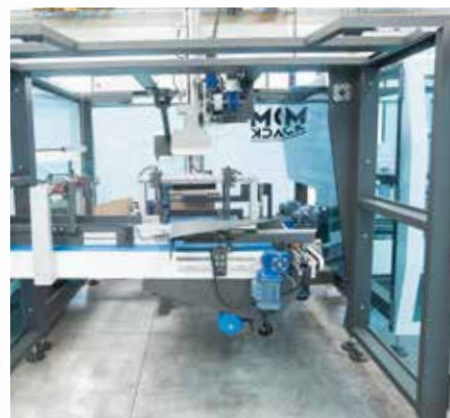
Completely accessible and openable. Loading and cartoning stations are separable to allow operator entering for easy maintenance.
